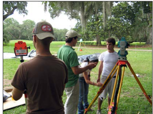
Figure 13: Training on the total station. Vertical control was maintained with the total station and with the manual transit, visible in the background
